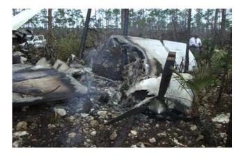
The aircraft hit several tall pine trees prior to making contact with the ground. It caught fire and exploded several seconds later. The aircraft was almost completely destroyed in the post impact fire.
