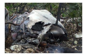
The engine sustained damaged due to the impact and was removed in joint participation with the Flight Standards Inspectorate and Teledyne Continental Motors. The engine was brought back to Grand Bahama International Airport to a secure storage area and later shipped for further evaluation to the experts of Teledyne Continental Motors.
