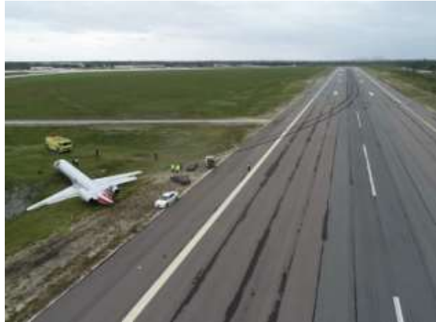
Fig.7 N674RJ tire signature markings on runway
